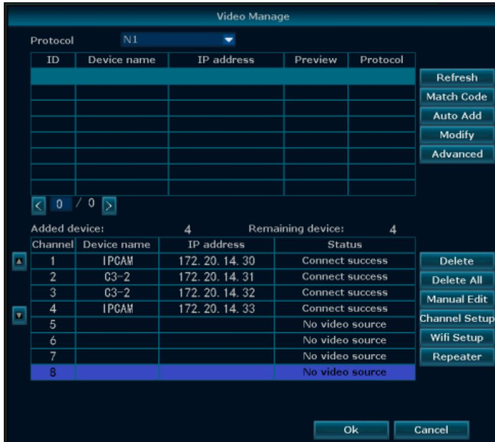
(2) Cam5 - 8 first paired with the IPC router connection (Connect up to 4-way), then in the Video Manage interface to search IPC Router, then click the "Auto Add" to add to the NVR.
