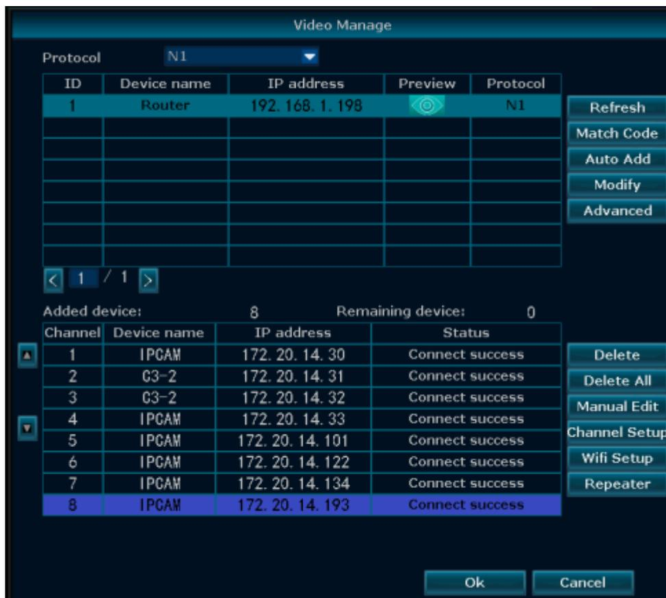
d. Click on the Repeater and the following is displayed. The green solid line of the Router indicates that the IPC router is wired connected .
